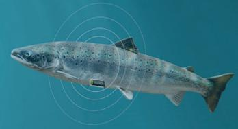
The Thelma Biotel DT transmitter is a low-power and versatile platform for depth and temperature measurements. It can measure down to 290 meters and can be made to present high resolution in any range of interest. The transmitter is produced in four different capsule diameters and with a wide range of battery packs, allowing optimization in size and operational life.
