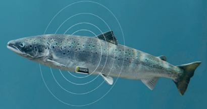
The Thelma Biotel depth sensors can deliver depth data down to 1000 meters and can be made to present high-resolution data in any range of interest. The depth sensor is available in all transmitter sizes and with a wide range of battery packs, allowing optimization in size and operational life. Two sensor types are available, the standard depth sensor, with a detection range down to 290 m, and the 1K depth sensor, with a range down to 1000 m.
