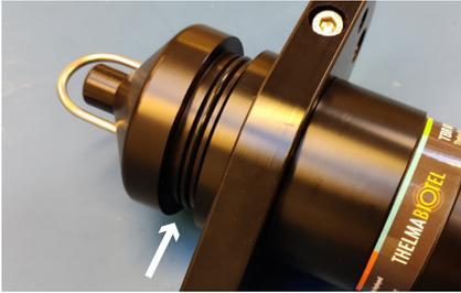
7. Check and lightly lubricate o-rings. Check sealing surfaces for damage or debris.
