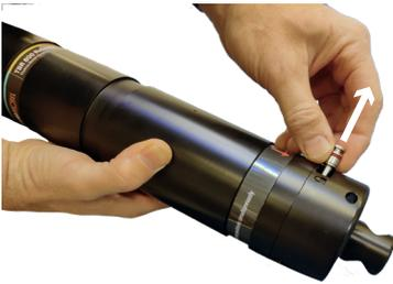
1. Remove key pin from locked deployment position. Use your finger, or any tool to pull out the edge of the key head located at the bottom of the receiver casing
