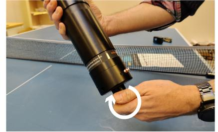
9. Insert the receiver into the casing and turn the release lug clockwise until the gap by the main o-rings is completely closed. Do not tighten with force.
