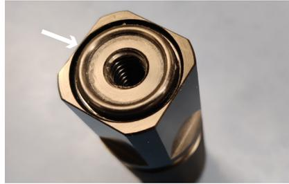
8. Remove the Key Pin from the unlocked service position and remove the release lug. Lightly lubricate the o-ring. Reinsert the release lug and the key pin into unlocked service position.
