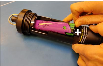
4. Pull the battery compartment clear of the casing and insert battery with plus towards the motor compartment. Ensure that the battery spring is compressed correctly while sliding the battery in and clicking it into place.
