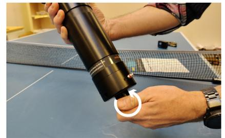
3. Turn the release lug counter clockwise to open and expose the battery compartment.
