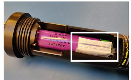
6. Put two humidity absorbent bags in the opening over the battery. Check the colour of the pellets for quality. Blue colour pellets are ready to deploy, white/translucent needs to be dried or replaced.
